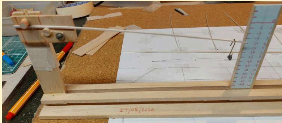
My jig for measuring deflection of the wing and prop spars.
