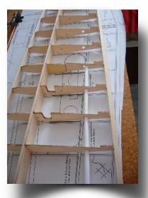
rather than the ply plates supplied. Unfortunately, huge schoolboy error, I fitted the bearers between the wrong ribs, so one bay out from where they should be. This did highlight to me, apart from what a muppet I am, how well the beech bearers were glued into the ribs. Now removed and fitted in the correct position.
