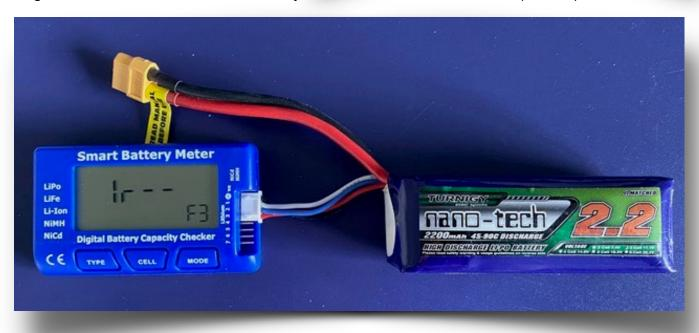
As the internal resistance increases with age and use, so the efficiency of the battery falls.
