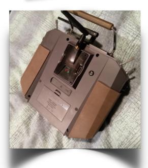
Finally here's a view of the back with the Jumper Multi-protocol module fitted. FrSky supply a blanking cover for this bay for when you don't have an external RF module in there. The Jumper module has red and green status LEDs, but they're not needed because everything they indicate can be found in more detail in the transmitter's settings/status pages:
