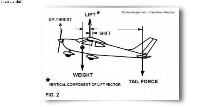
**D**/ Note that as the nose goes up, the nose-heavy moment distance reduces slightly, reinforcing the effect of Centre of Pressure shift.
