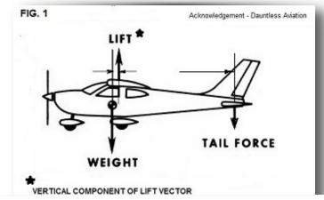
If we now grossly increase nose-weight, then we have to set up-trim at the elevator to provide greater balancing down-force there. This now comes to the nub of the question - why does the model fly nose-up in this condition, and not just fly level with exaggerated elevator up-trim applying this additional force?
