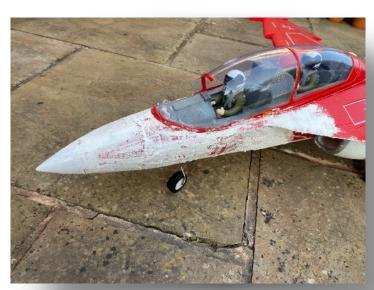
13. As already stated, expanded foam can give a bubbled-up appearance, so a layer of filler applied over the area, then sanded down, can help achieve a smoother surface.
