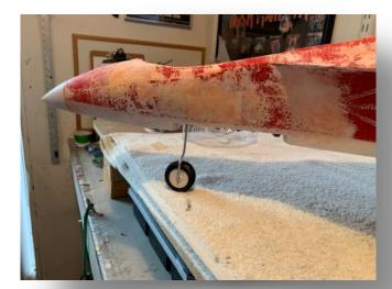
15. Repainting comprised several coats of colour-matched matt emulsion from B&Q (Valspar). As an aside, B&Q is a great source of touch-up paint in general; all that's required is sample of the original colour and for just £3 the nice folks there will mix a good-sized tester pot which is a perfect match. The only decision to make is whether you want silk or matt.
