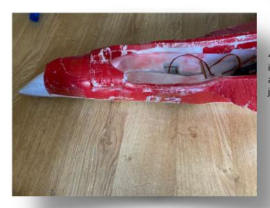
4. If there are parts that fit together well, even if crushed, stick them together with a suitable adhesive; I use epoxy, but other foam glues work just as well.
