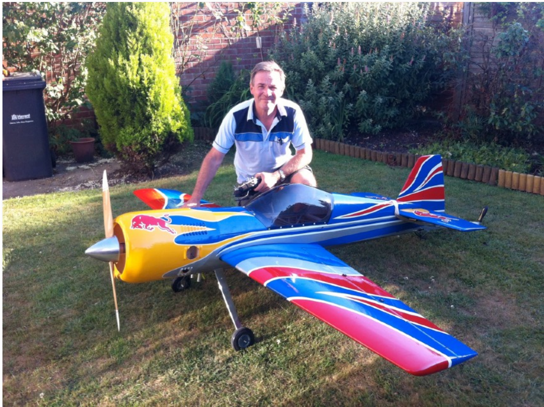
Duke Benson's Wild Air SU26 in Red Bull Markings The engine is a DLE 110cc two stroke twin petrol engine it has a wingspan of 103inches (2.69 metres) and weighs 27lbs
