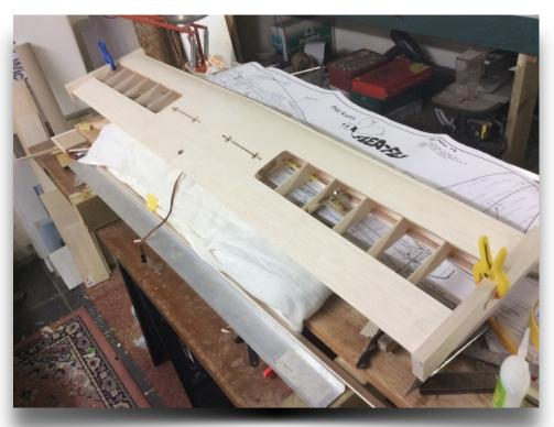
The wing is very strong with spruce spars, built upside down and using a single servo with snakes substituted for piano wire. Do not forget to turn the wingover when joining for the small amount of dihedral required. The ailerons are cut out after sheeting is finished.
