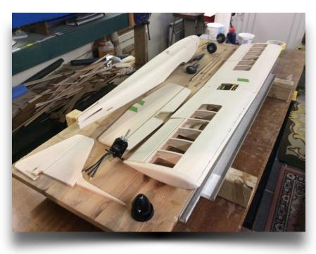
Covering was to be film for the wings, tail plane and initially the fin. I gave up on the fin and decided to paint it. This could be another story as the fin took two weeks to finish etc. The fus is glass sheathed with epoxy (eventually the fin) and painted with Humbrol Acrylic spray paint.
