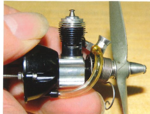
Go down a size to the Cox .010 (0.163cc) and you'll need to strain the fuel through your handkerchief and then a paper coffee filter.
