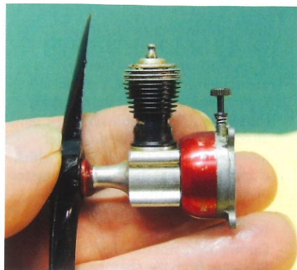
Imagine the size of the fuel jet hole in this little Cox .020 - the need for super-clean fuel is obvious.
