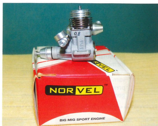
The Norvel range were real screamers - very high rpm, but the smallest foreign matter in the fuel feed cut them dead almost instantly.
