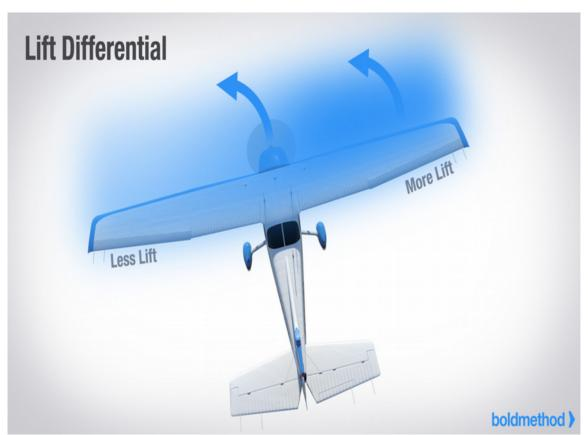
And at the same time, your low wing produces more drag, because it's at a higher angle-of-attack. And that drag causes your plane to yaw into the spin. When you combine both forces, you wind up in a fully-developed spin.
