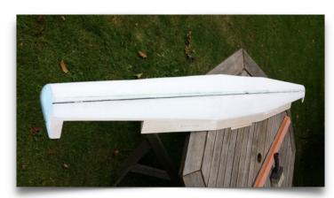
(i.e. they are part of the wing section) not Fowler flaps as on the full size. Fowler flaps are easy enough to make, but you end up with huge hinge fences under the wing, which doesn't look good. They are 1/16" balsa sheet, hinged with the medical. The ailerons are balsa TE section cut to size and hinged the same way. The servos are let into the bottom of the wing with just the actuating arm sticking out.
