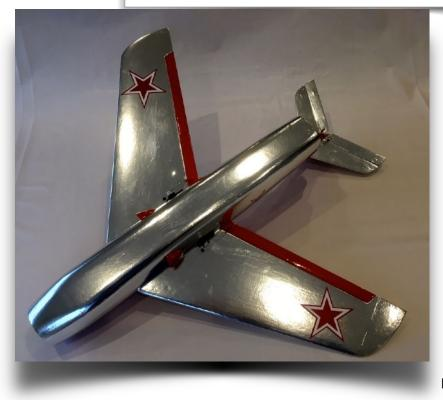
I made a big mistake when I started covering the shiny bits with 'Fibre Film' which has no adhesive backing. I foolishly painted 'Balsa Lock' on to the wood....which caused the wood to swell up and go grainy...so I had to wait for it all to dry and harden before I could sand the whole lot down again. Having applied it on the reverse of the film I had no further difficulties with the main covering although it is far less pliable that normal film.
