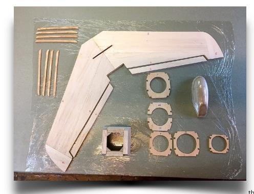
I chose my normal route of tracing the formers and ribs from the plan and then photocopying them and sticking them to the wood with Prit Stick before cutting, and I applied the 'Tony Reynaud' method of forming the canopy from a pop bottle. TN does, however, provide a laser cut parts service and pre-formed canopy if required.
