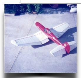
Towards the end of the last century, 1973 to be exact, I designed a Control Line Stunt model based on the American Corsair Fighter. At 72" span, it was big for a C/L model but the old Merco 61 was powerful enough to keep the lines tight on overhead manoeuvres.
