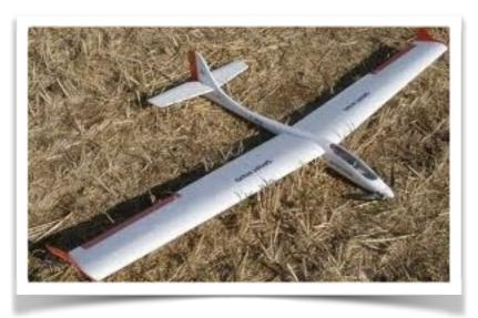
by a MVVS 3.5/1200 Sport Brushless Motor turning a  $12 \times 6$  folding prop, the EMF comes a 2.300 3s Lipo.
