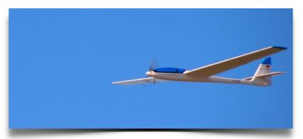
The Mistral has been built to utilise rudder, elevator, ailerons and throttle functions, with a coupled rudder and aileron option, I declined to fit the optional air-brakes. The wings, tailplane and rudder were covered with white Oracover and the fuselage was polished with Rubbing Compound and T Cut to remove the mould join and left white. The colour scheme being loosely based on German full size gliders, the transfers being made on a computer.
